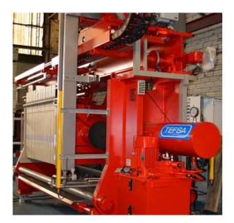
The cable overhead PSEH filter presses have been designed with a transport system which does not require any greasing. This makes them highly suitable for very corrosive environments such as acid industry, metal refineries and clean environments such as food industry, pharmaceuticals, oil refining, greases, agar and carrageenan, among others.
