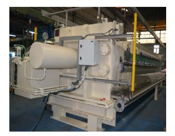
EHPT is a sidebar filter with reciprocating plate transport system. Its design with four rods to join the two frames gives it a very high resistance and avoids the filter pack deformation, which is a very usual effect on automatic sidebar filters when the pressure is high, especially with membrane plates.
