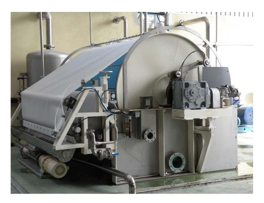
The drum filter is another type of continuous operation filter. The main difference in this case is that it allows different types of discharge systems according to the filtrated product.
