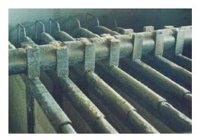
Leaf filters are suitable for low solid concentration products, high temperatures, easily oxidizable products, dangerous or polishing filtrations with precoat.
